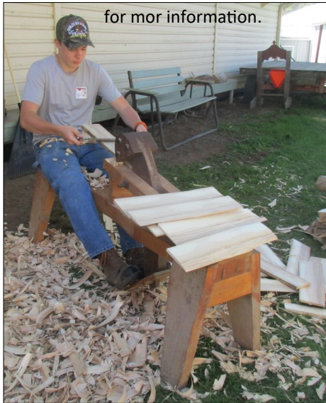
A group of misfits, as they call themselves, got together to demonstrate how to make shake shingles, the most popular roof material in the 1800's. Ben Deuschle and Lucas Drever
